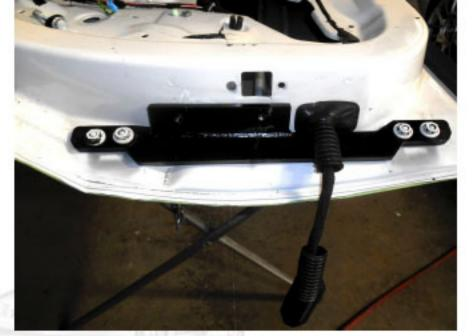
One the bracket is securely installed on the door now you can install the second section of the now VDI hinge system.
