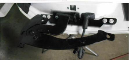
Once the two pieces of the hinge and securely connected you can install the new VDI hinge on the car. Make sure to use a helper. Make sure that all the factory marks are on the correct position and the distance from the apron and the edge of the doors is the correct one.
