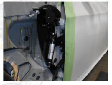
Asked your helper to raise the door and installed the shock as shown on the image on the right.
